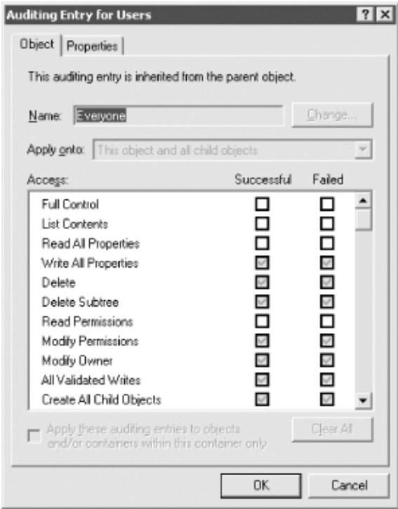
Figure 11-13 shows an example AE window for successful and failed auditing of properties. Here you are auditing only property writes.
